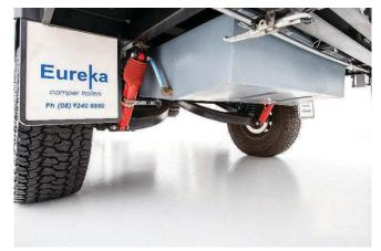
2 Tonne rated Independent Dobinson coil spring suspension, Pedder shock absorbers, hydraulic disc brakes & 110 L water tank
