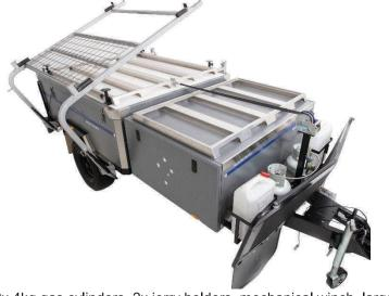
2x 4kg gas cylinders, 2x jerry holders, mechanical winch, large stone guard and offroad hitch. Optional gas strutted boat loader
