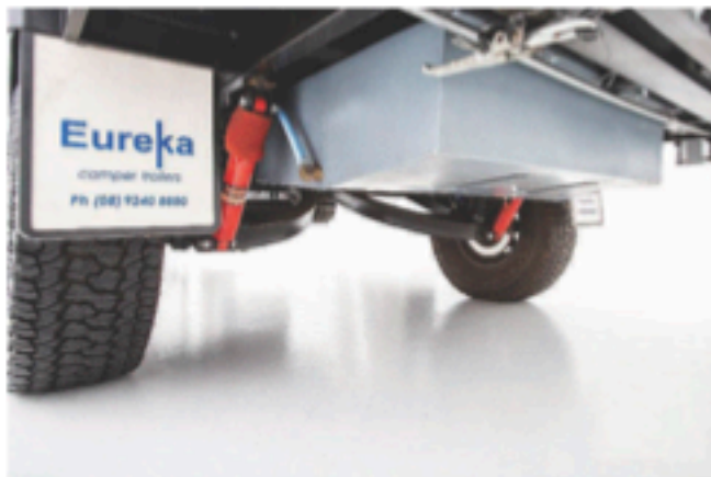
2 Tonne rated Independent coil spring suspension, Pedder shock absorbers, hydraulic disc brakes & 110 L water tank
