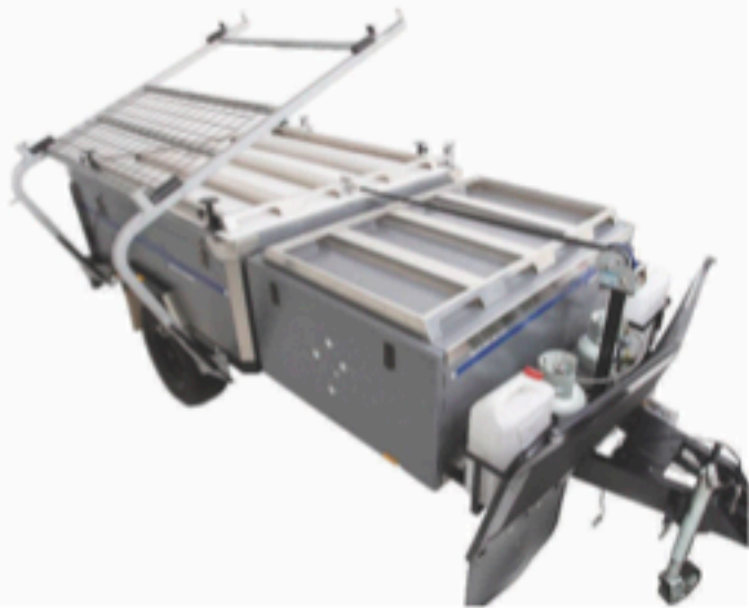
2x 4kg gas cylinders, 2x jerry holders, mechanical winch, large stone guard and treg hitch. Optional gas strutted boat loader
