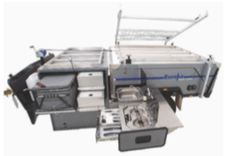
Kitchen with sink, 3 burner cooker, cutlery drawer, table, double pantry, and sliding drawer to take 60L Engel fridge/freezer
